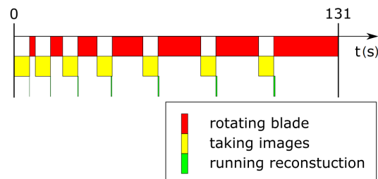
Figure 11. Time line of density reconstruction with N_a = 7 projection measurements. The angles are chosen such that more projections are acquired in the direction parallel to the shock front, maximizing the information about the shock. For each projection 20 images were acquired, 10 of which were recorded with the gas jet on and the other 10 with the gas jet off, as a reference.
