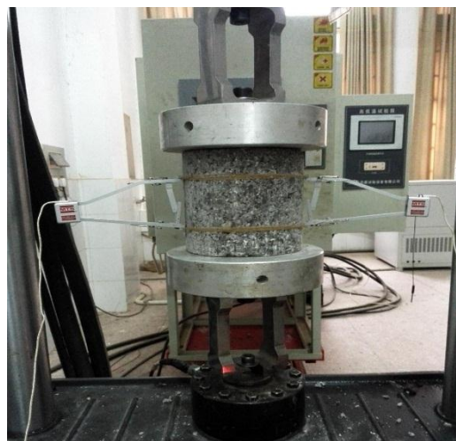
Figure 6. Device of compression resilience modulus test.
