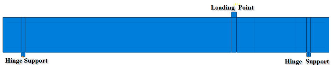
Figure 15. Proposed numerical model for concrete slabs.
