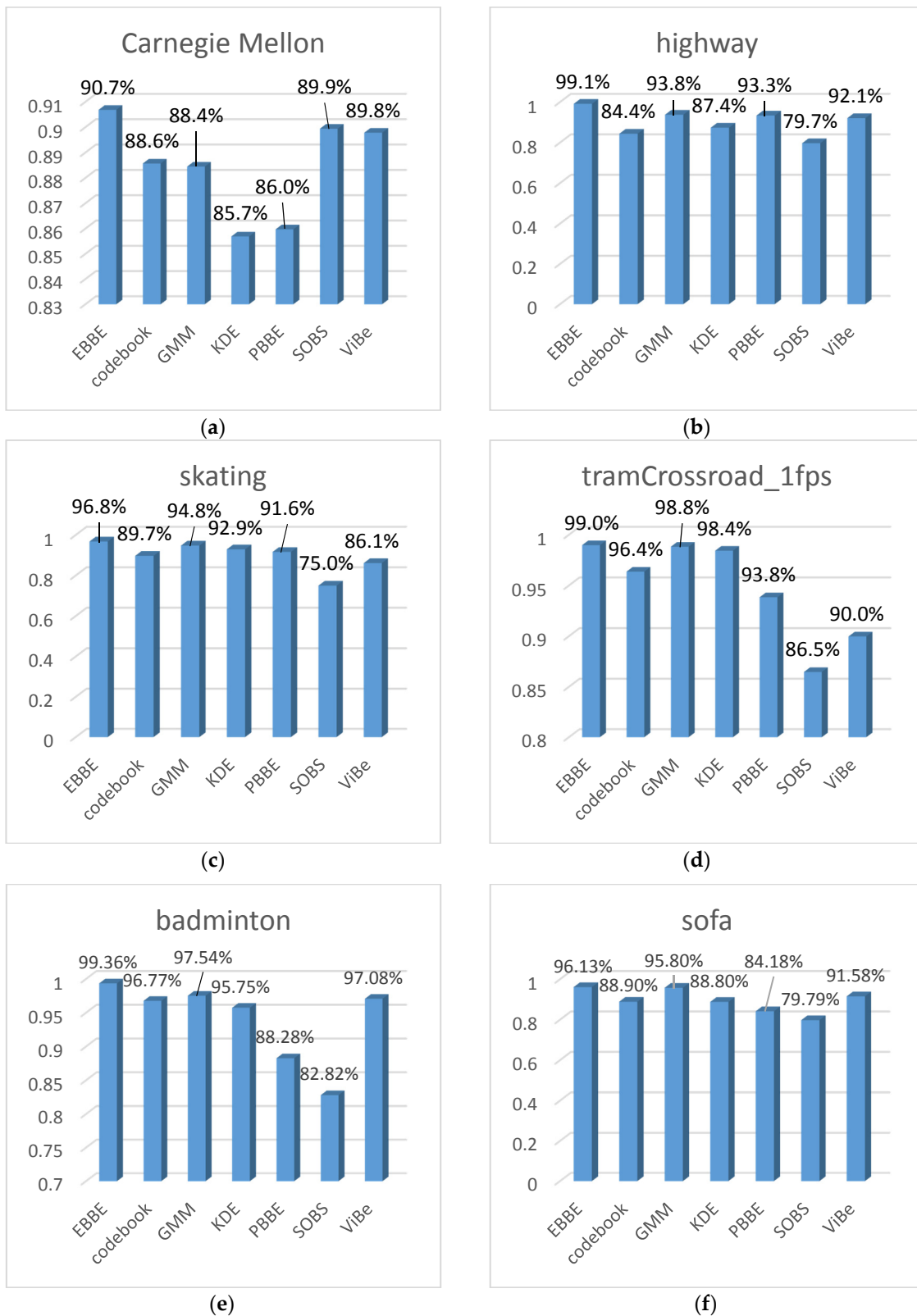
Figure 13. PCCs of seven background subtraction methods. (a) Results for the sequence (Carnegie Mellon). (b) Results for the sequence (highway). (c) Results for the sequence (skating). (d) Results for the sequence (tramCrossroad_1fps). (e) Results for the sequence (badminton). (f) Results for the sequence (sofa).
