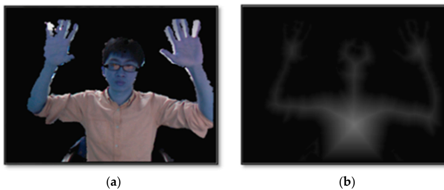
Figure 5. The distance transform process to highlight the outline of a skeleton frame: (a) before distance transform and (b) after distance transform.
