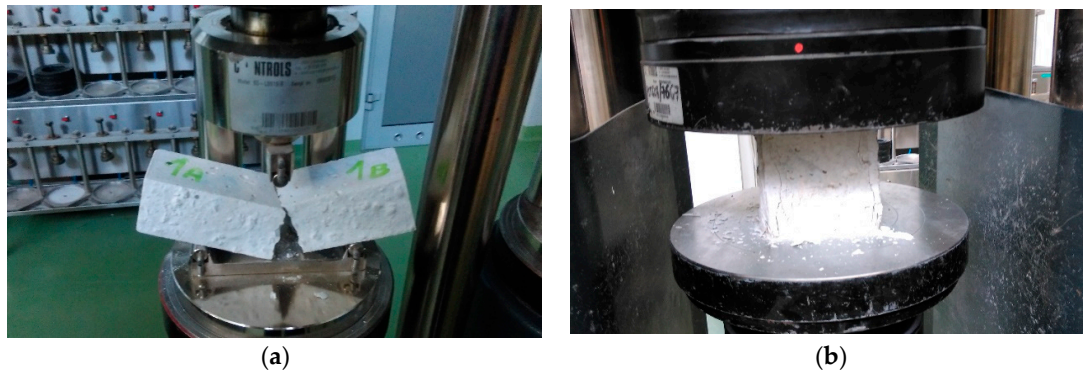
Figure 4. Example samples used in the research: (a) beam sample; (b) cubic sample.
