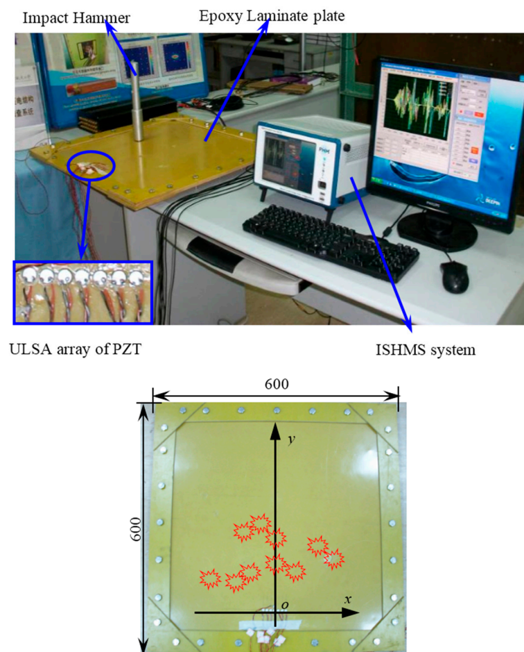
Figure 3. Experiment setup, ULSA arrangement, and impact applied positions (mm).
