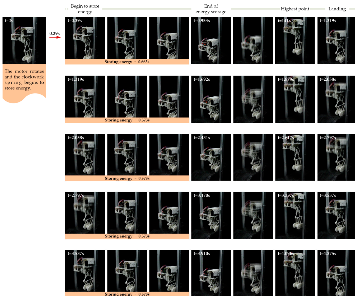
Figure 16. Experimental process of hopping performance test.
