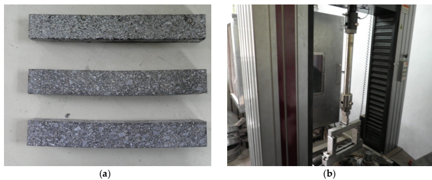
Figure 12. Three specimens (a) and Materials Testing System (MTS) (b) for low temperature bend test at -10\text{ }^{\circ}\text{C} , at loading rate of, 50 mm/min.
