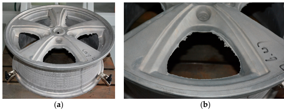
Figure 11. Casting blank of automobile hub: (a) overall appearance of automobile hub; (b) disc burrs of automobile hub.
