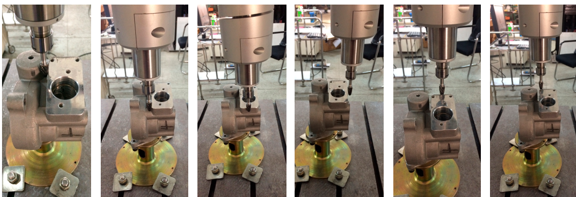
Figure 23. Experimental deburring of facet edges on top facet.
