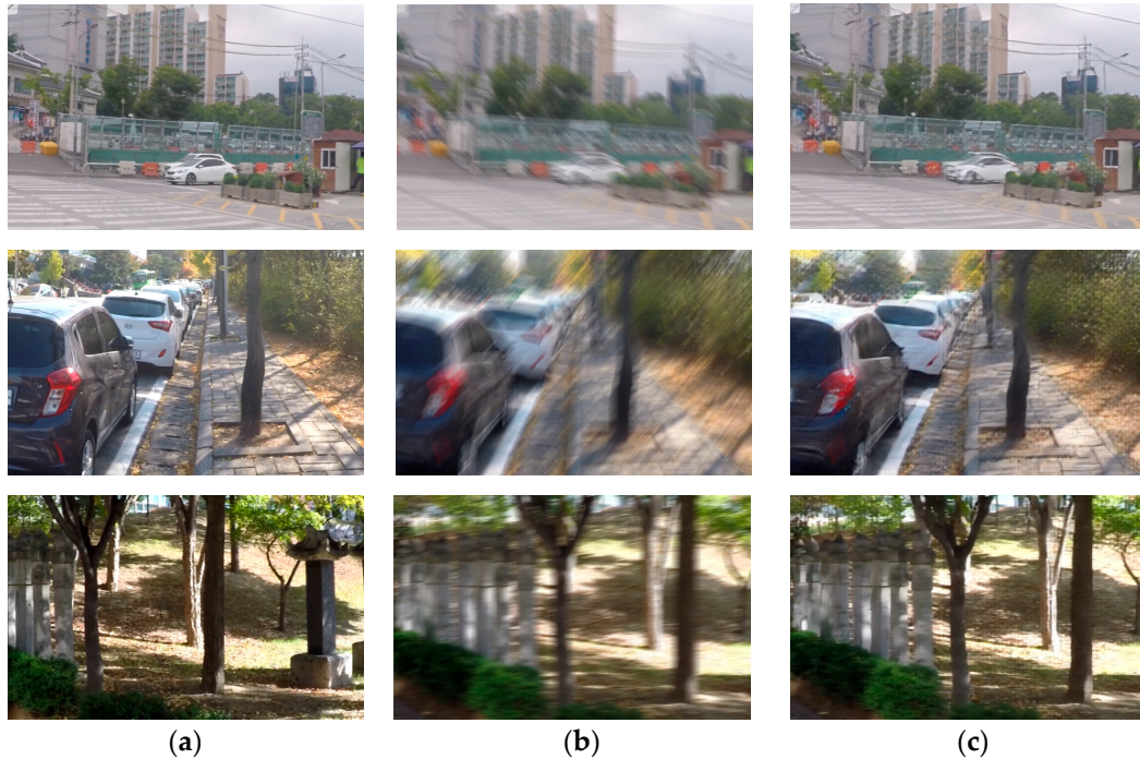
Figure 8. Example images of WGAN-GP with content loss function: (a) Sharp image. (b) Blurred image (c) Reconstruct image.
