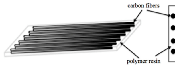
Figure 1. A typical structure of carbon fiber reinforced polymer (CFRP).
