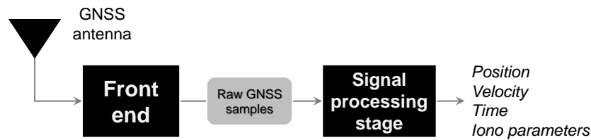
Figure 2. Generic architecture of a Software Defined Radio (SDR) satellite navigation receiver.
