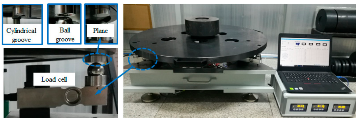
Figure 13. Experiment platform for measuring mass and CG.
