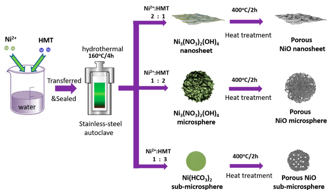
Figure 6. The synthesis route of hydrothermal reaction and subsequent calcination for mesoporous NiO hierarchical nanostructures.
