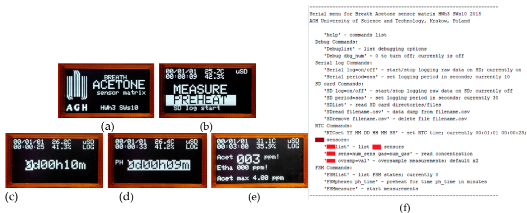
Figure 5. User interface screens of the developed portable gas analyzer. Splash screen (a), main menu (b), preheat setting (c), and executing (d) measurement screen presenting the acetone concentration and the raw data from each sensor (e). Alternatively, the analyzer can be controlled through a serial interface (f).
