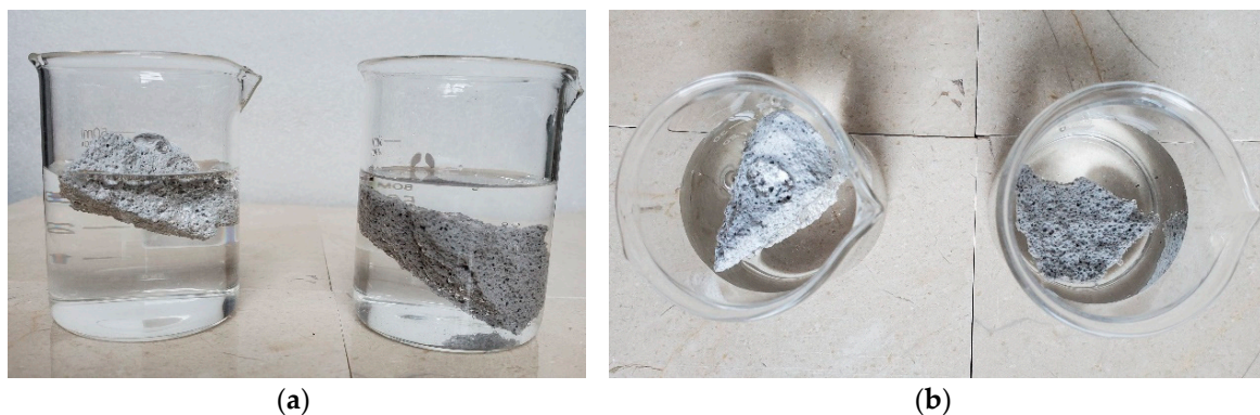
Figure 8. Water immersion experiment of the aerated bricks w/o surface modification: (a) Side view; (b) Top view.
