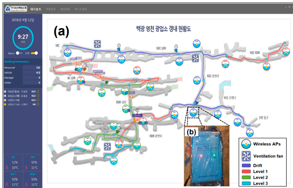
Figure 2. Components of the mine safety management system installed in the study area: (a) main dashboard showing the location of dump trucks and loaders; (b) wireless APs.
