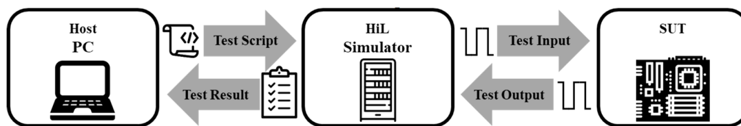
Figure 2. Hardware-in-the-loop (HiL) test environment.
