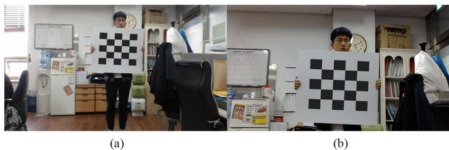
Figure 4. Camera calibration process for extracting RGB camera internal parameters and acquiring distance difference between RGB camera and HoloLens camera. (a) RGB camera picture; (b) HoloLens camera picture.
