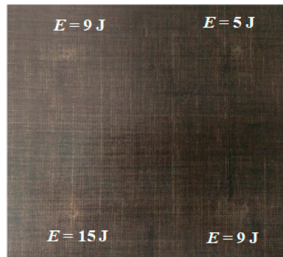
Figure 4. Photo of the polypropylene added with 2% maleic anhydride (PA6B) specimen with indicated energy and location of the impacts.
