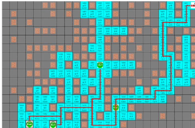
Figure 14. The simulation result of A* algorithm for the fourth situation.
