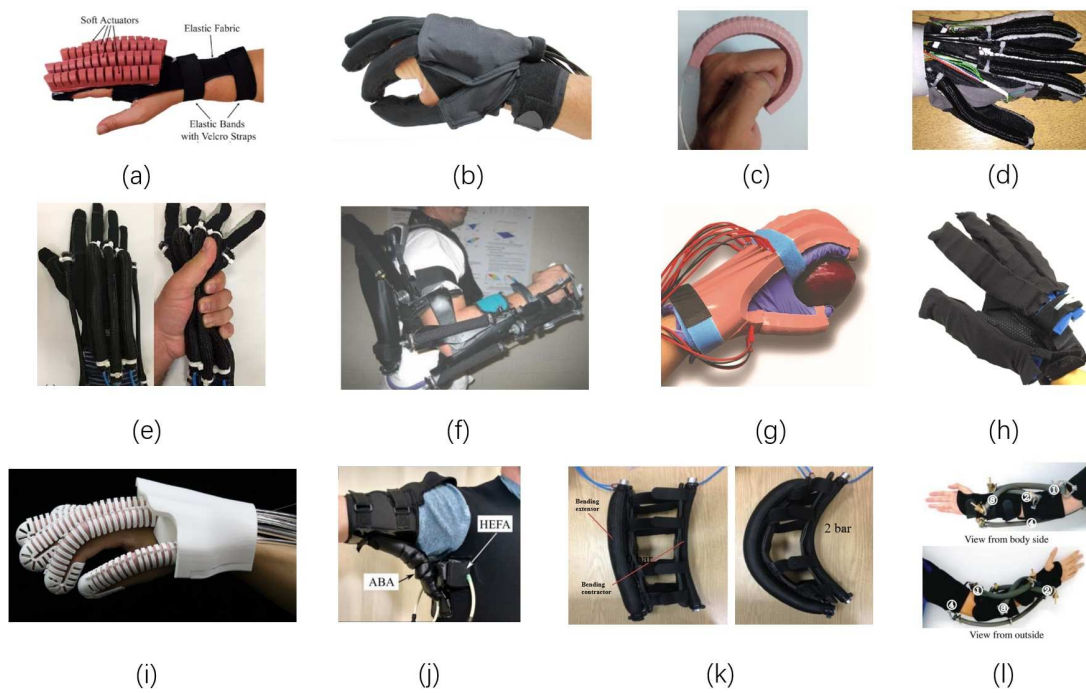
Figure 3. Soft rehabilitation and nursing-care robots based on pneumatic fiber braided fabrics and elastic polymers in upper limb. (a–d) is reprinted from [49,52,53,55], respectively. (e–h) is reprinted from [56–58,62], respectively. (i–l) is reprinted from [64,67–69], respectively.
