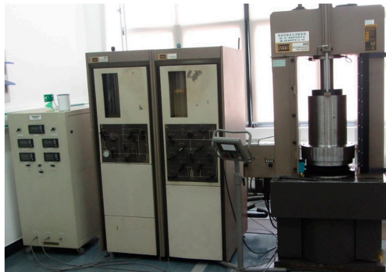
Figure 2. MTS 815.02 Electro-hydraulic servo-controlled rock mechanics testing system.
