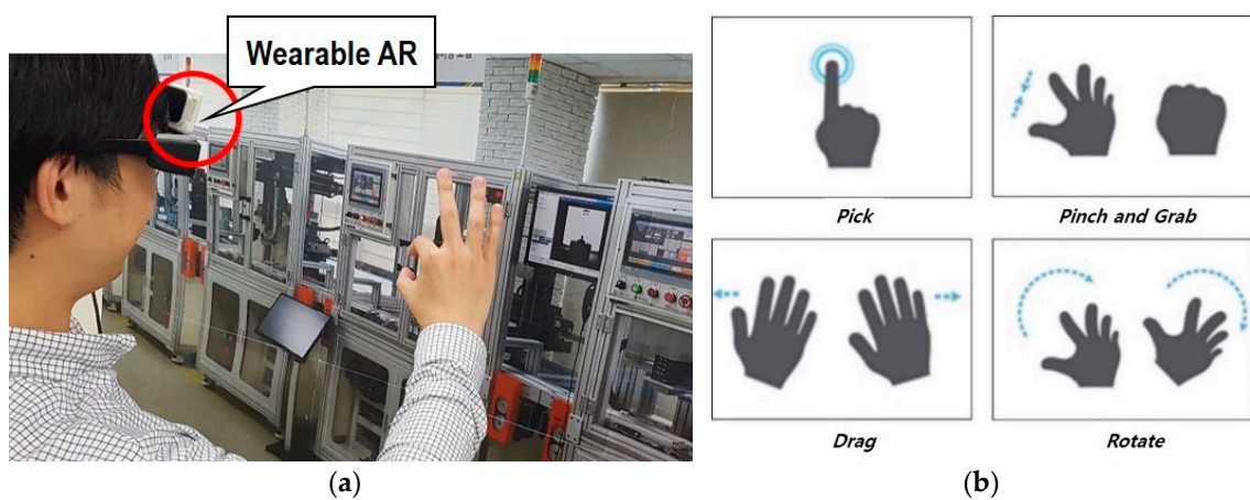
Figure 6. Hand gesture-based interaction (a) in wearable AR for monitoring a manufacturing service; (b) different types of hand gesture interactions.
