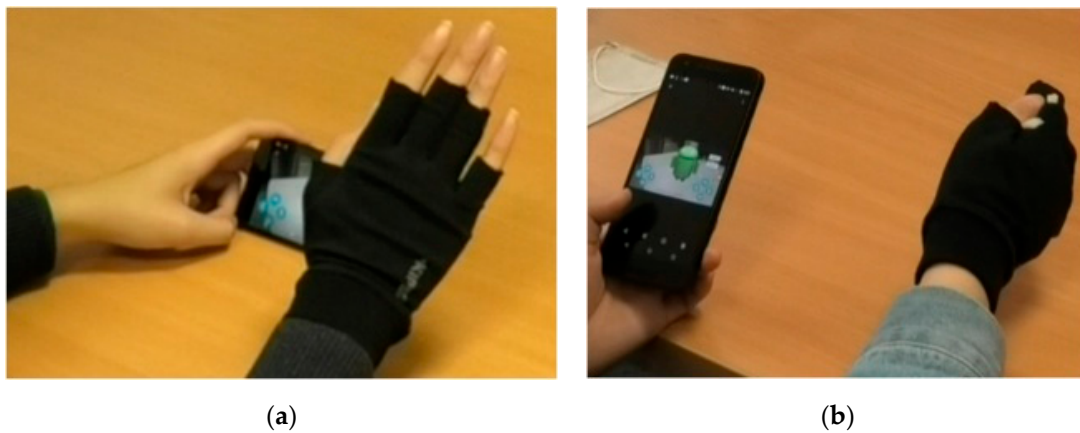
Figure 3. Variety of gestures performed by our participants using one hand (right hand) while holding the device on the other hand: (a) wrist gestures and (b) thumb-to-index touch gestures.
