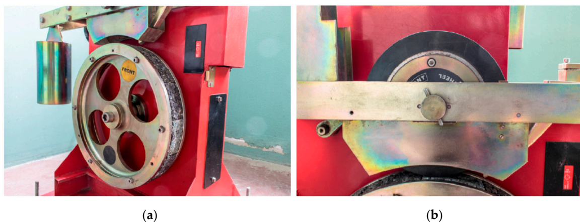
Figure 4. Accelerated polishing machine: (a) revolving wheel; (b) polishing tire-wheel by corn emery.
