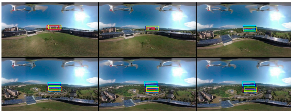
Figure 11. Tracking results on 360-degree video sequence 8 (tracking windows with different colors: MOSSE MIL MedianFlow BOOST TLD KCF GOTURN CSRT).
