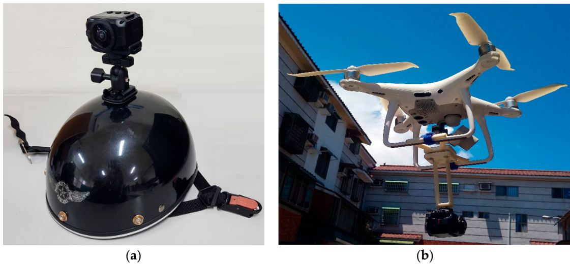
Figure 2. Two ways to set up an omnidirectional camera: (a) installed on top of a helmet for ground video capturing, (b) attached to a drone for aerial video capturing.
