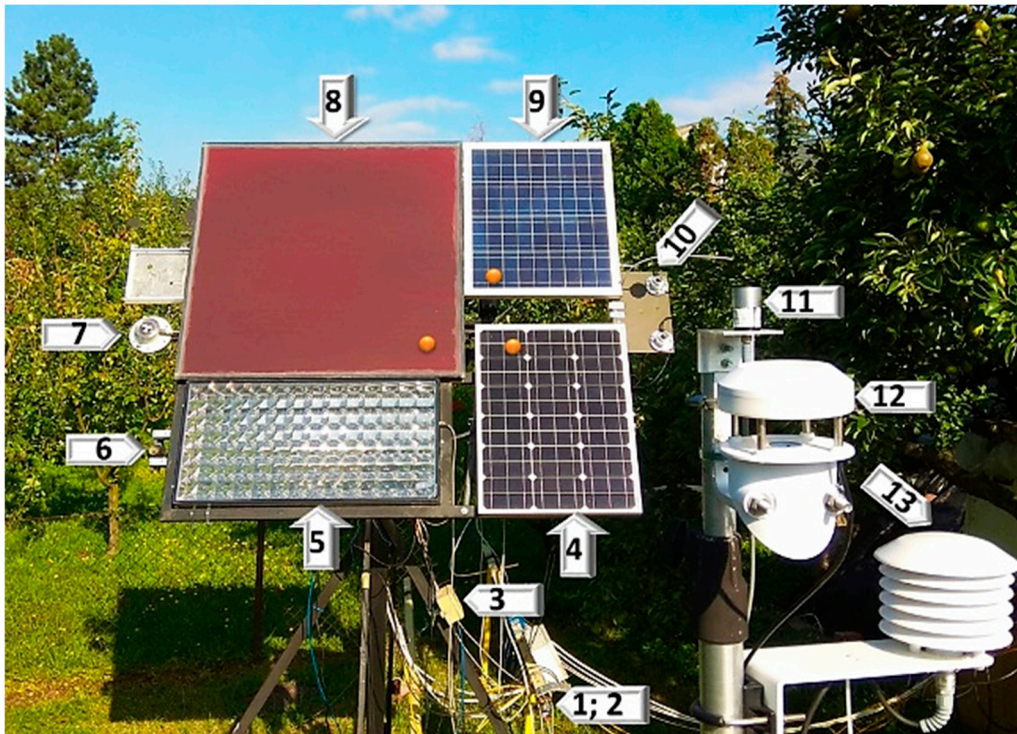
Figure 3. The measuring station in Keszthely (1, HYTE-ANA-1735 humidity module [measuring air humidity]; 2, Pt 100 sensor; 3, manual/automatic tracking control unit; 4, m-Si module; 5, CPV module; 6, photosensors; 7, Eppley Black and White pyranometer; 8, a-Si module; 9, p-Si module; 10, Hukseflux LP02 pyranometers; 11, EMS 11 Silicon PV detector; 12, DS-2 Sonic anemometer; 13, OTT TRH relative humidity sensor; Orange dot: Pt 100 sensors).
