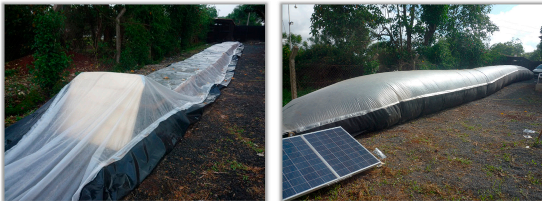
Figure 1. Inflatable solar dryer (ISD) before being inflated (left, note the deflector board) and the inflated ISD during drying experiments (right).
