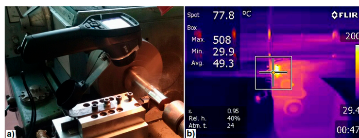
Figure 1. Experiment setup: (a) a view of the thermal camera when measuring, and (b) a thermal imaging with measurement position.
