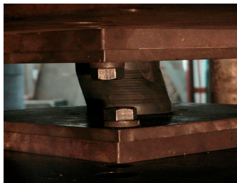
Figure 3. The rubber bearing in testing.
