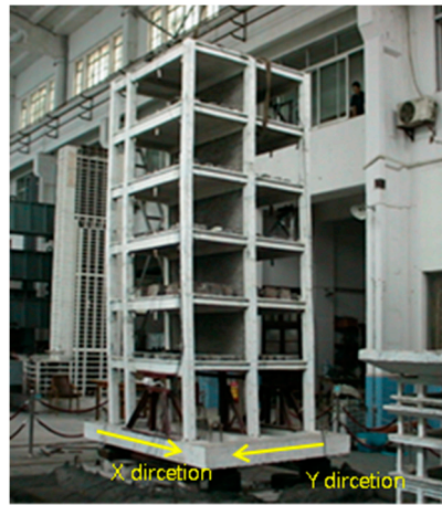
Figure 2. Six story reinforced concrete frame structure.
