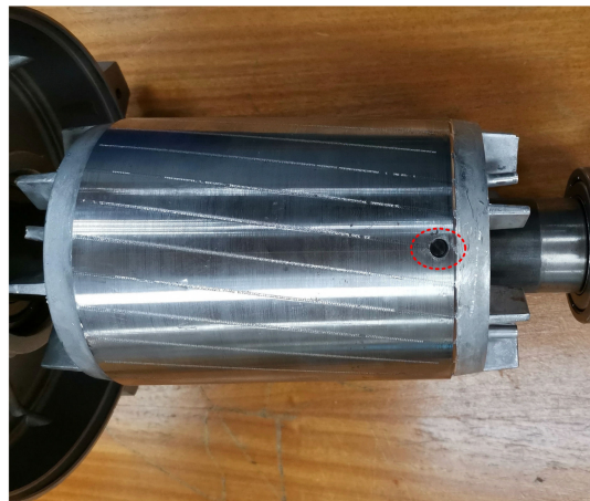
Figure 9. The faulty rotor simulated with one bar breakage.
