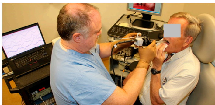
Figure 12. Illustration of a clinician holding a left-handed ISP probe that is designed to measure the left vocal fold collision pressure. The clinician's right hand operates a standard camera sensor for standard video or video stroboscopic imaging.
