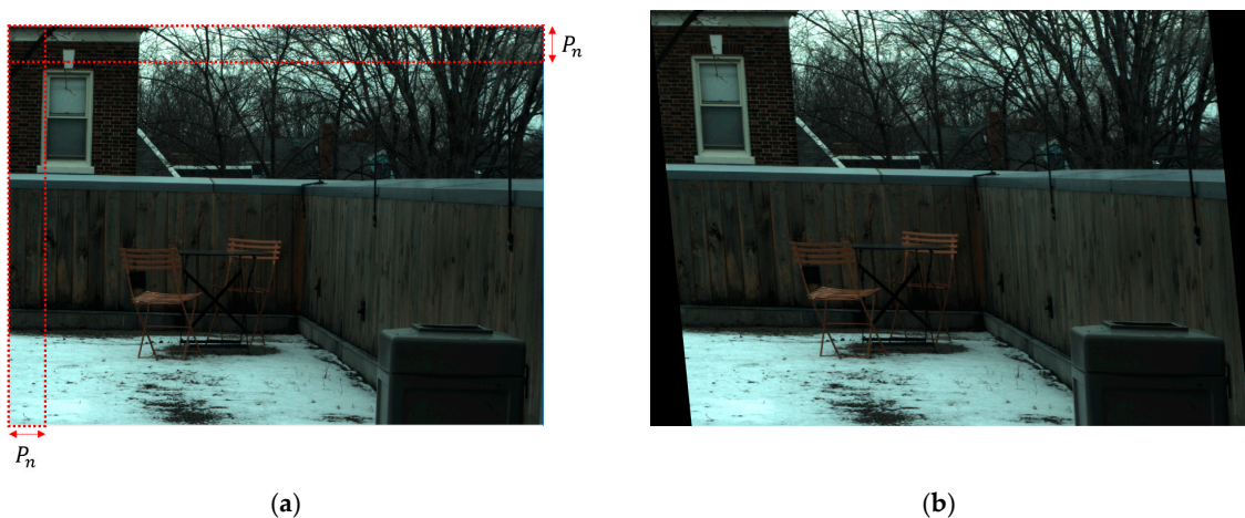
Figure 5. Example of pixel mismatch representation using (a) cutting off ( P_n indicates the number of pixels cut off from the left and upper sides) and (b) shear transformation.
