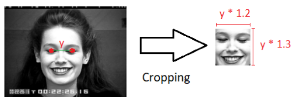
Figure 9. Background removal using the distance between eyes of a face from the CK+ database.
