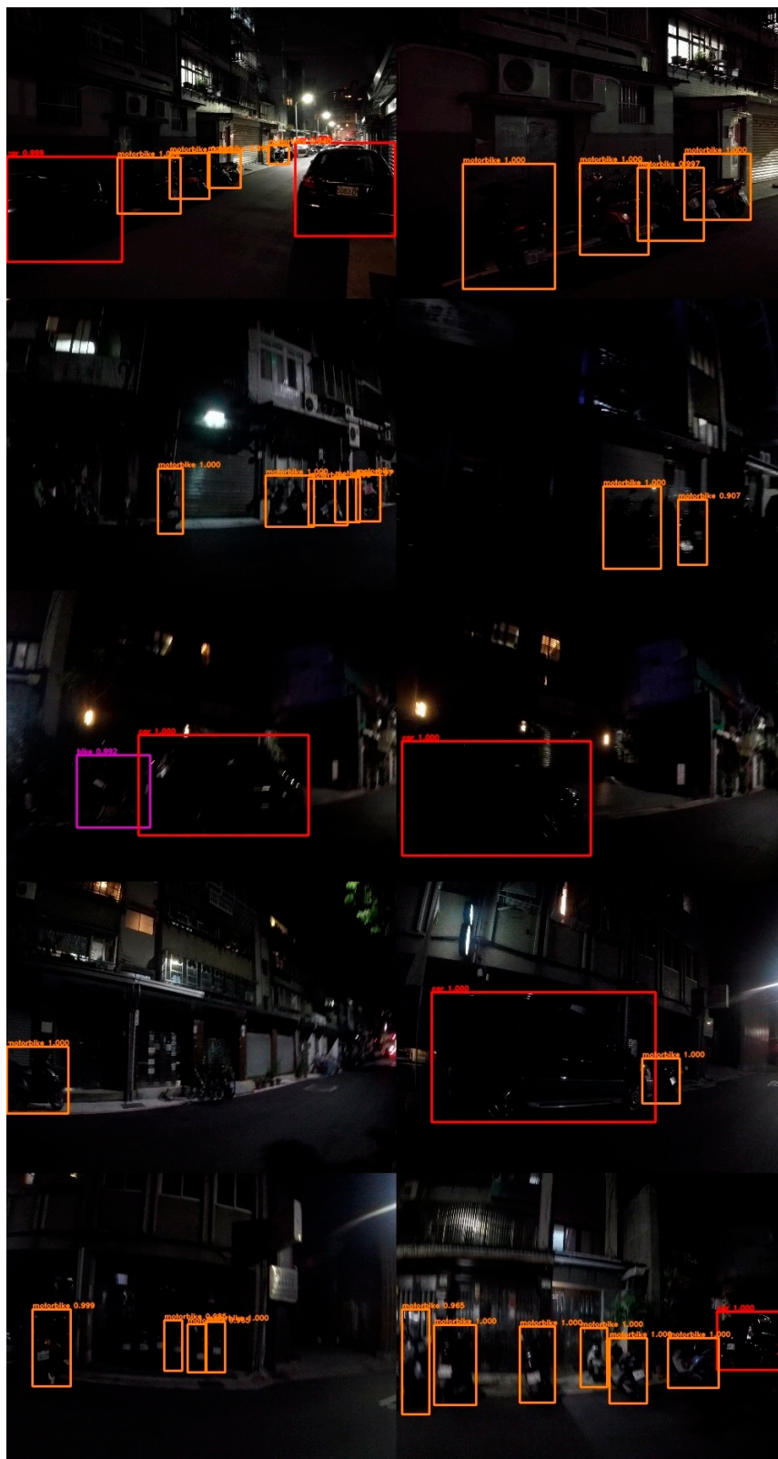
Figure 25. Outputs from the Faster R-CNN [5] with ResNet101 [2] in our proposed system trained using our nighttime data.
