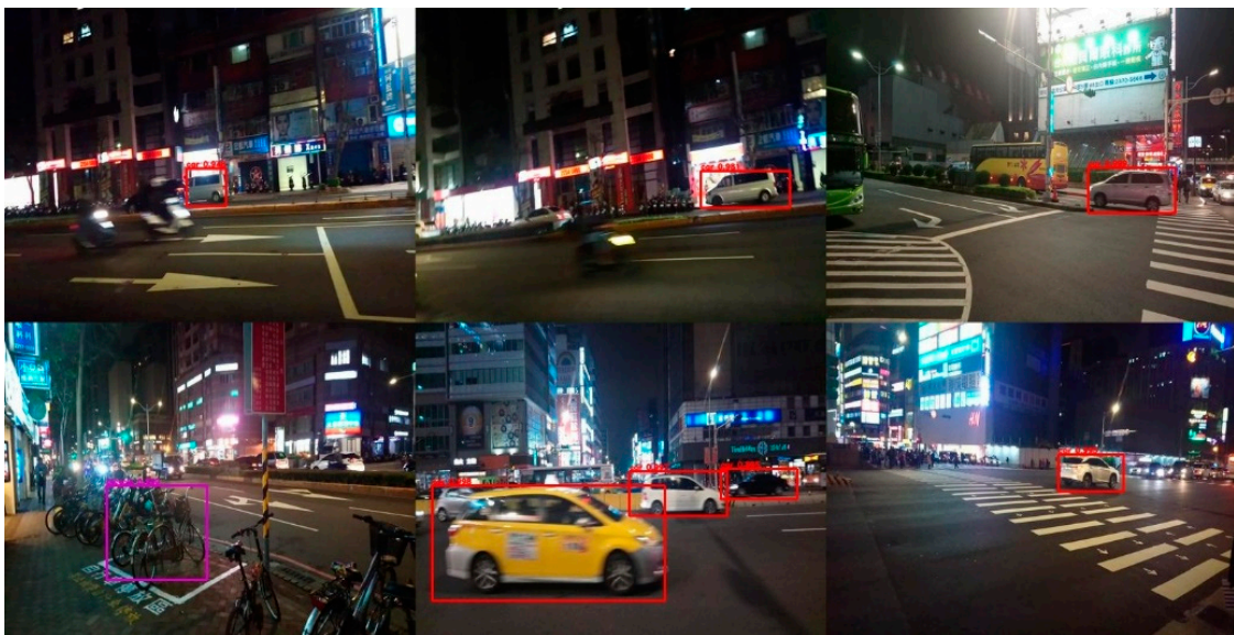
Figure 1. Urban nighttime images processed by the Faster R-CNN [5] with VGG16 [1] trained using PASCAL VOC 2007 [6].
