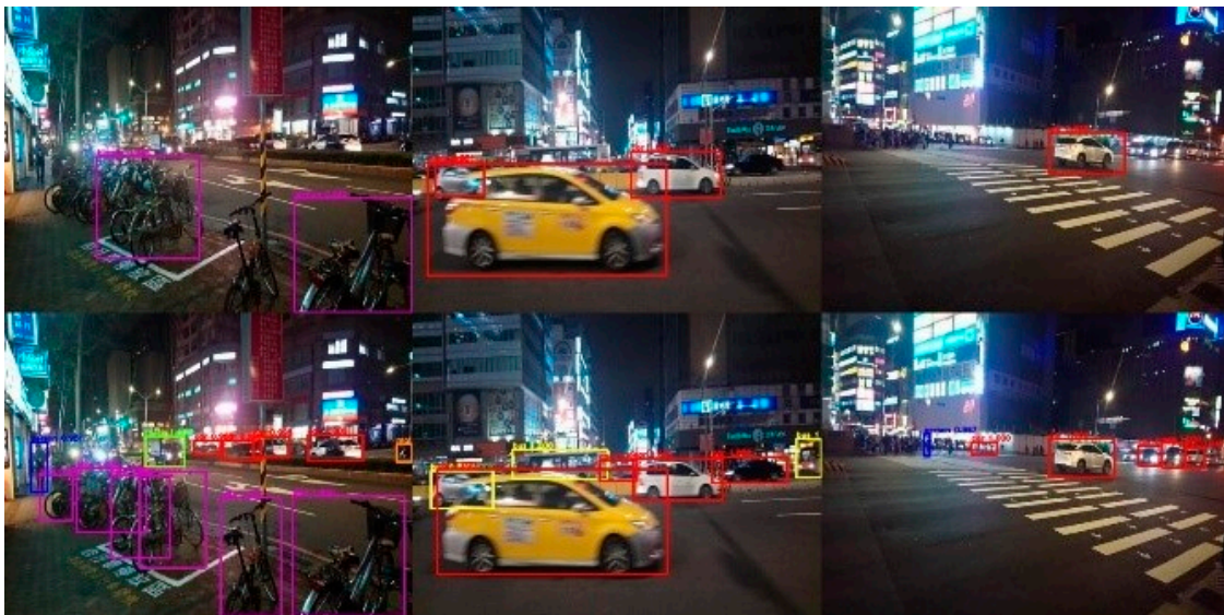
Figure 21. Outputs from two variants of the Faster R-CNN [5] with ResNet101 [2]. Upper row: Ordinary model trained with PASCAL VOC 2007 [6]. Lower row: Proposed system trained with our nighttime data.
