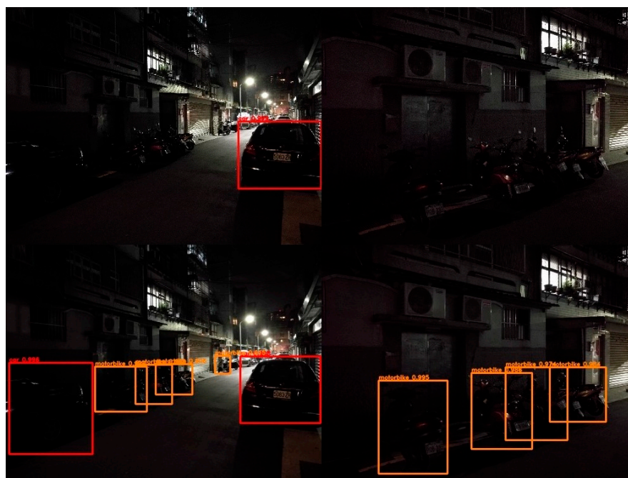
Figure 3. Extremely dark images processed by the Faster R-CNN [5] with VGG16 [1]. Upper row: Trained with PASCAL VOC 2007 [6]. Lower row: Trained with our nighttime data.
