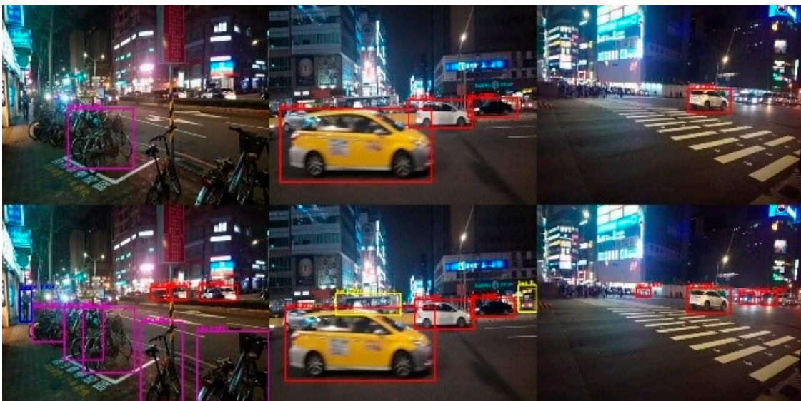
Figure 19. Outputs from two variants of the Faster R-CNN [5] with VGG16 [1]. Upper row: Ordinary model trained with PASCAL VOC 2007 [6]. Lower row: Proposed system trained with our nighttime data.
