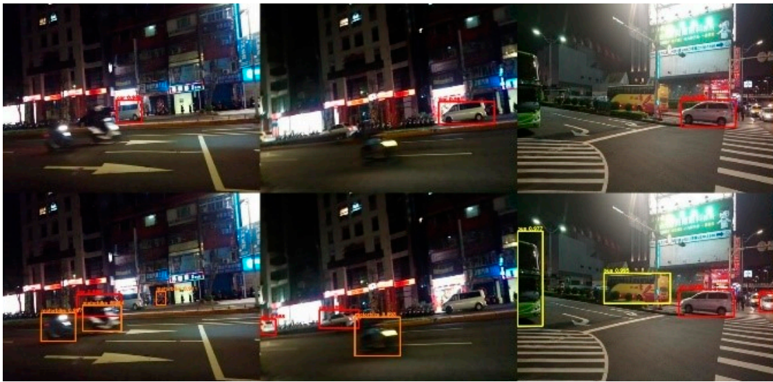
Figure 18. Output from two variants of the Faster R-CNN [5] with VGG16 [1]. Upper row: Ordinary model trained with PASCAL VOC 2007 [6]. Lower row: Proposed system trained with our nighttime data.
