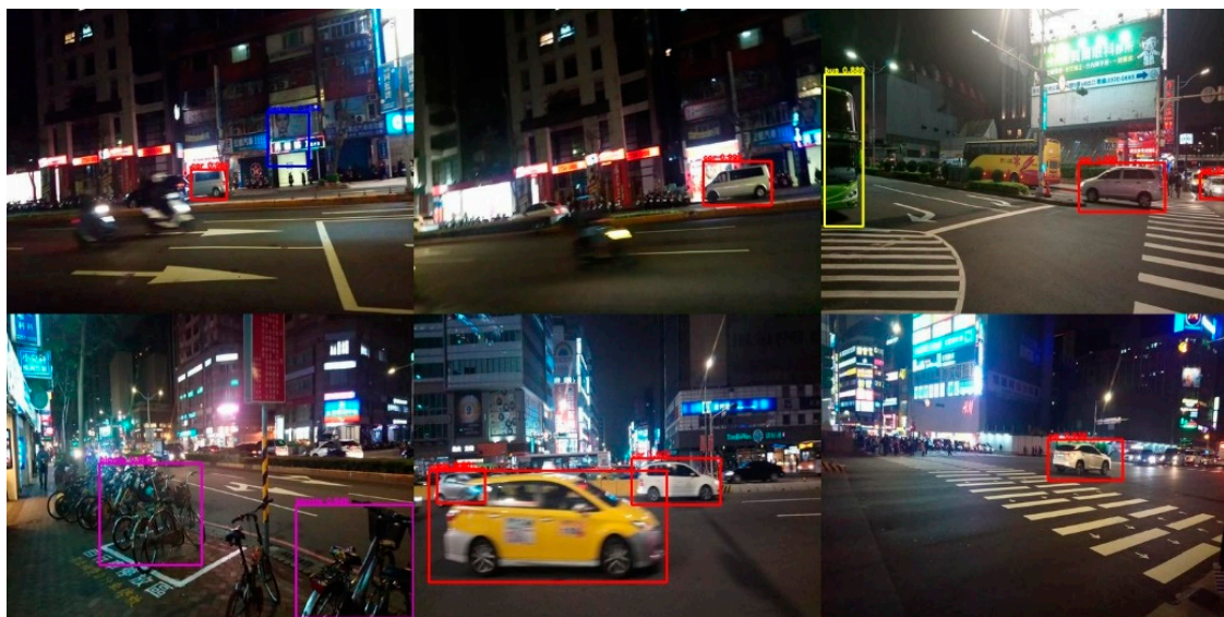
Figure 2. Urban nighttime images processed by the Faster R-CNN [5] with ResNet101 [2] trained using PASCAL VOC 2007 [6].
