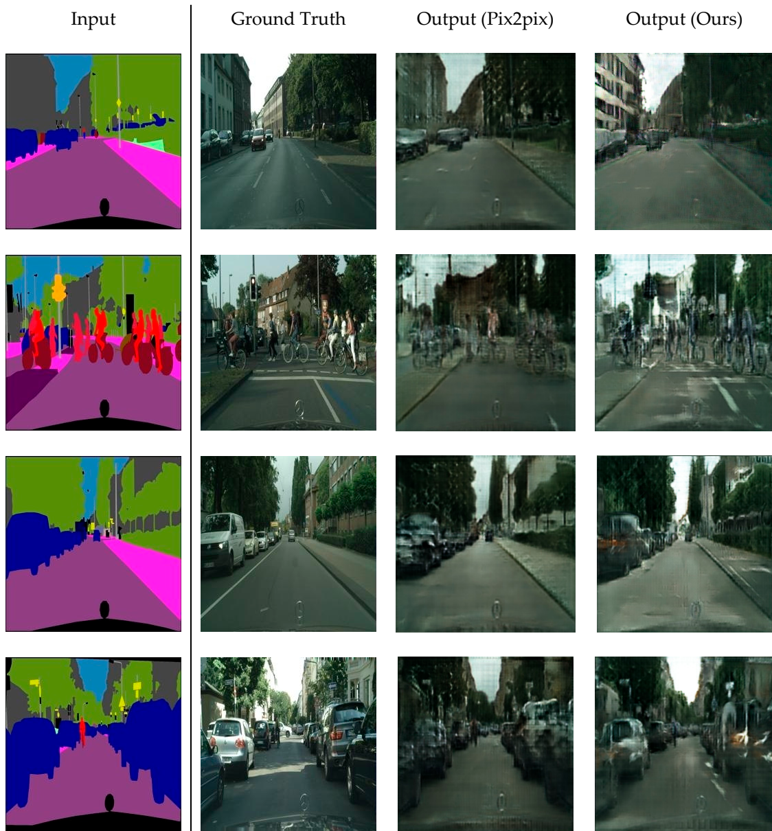
Figure A1. Comparison of Pix2pix and our model. The introduction of noise, including mixed textures, faded edges, and blurred objects, are mitigated in our model.
