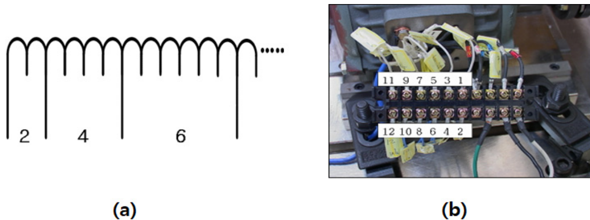
Figure 8. Method for configuring artificially turn short: (a) short of stator winding (b) external tab of the turn-short motor.
