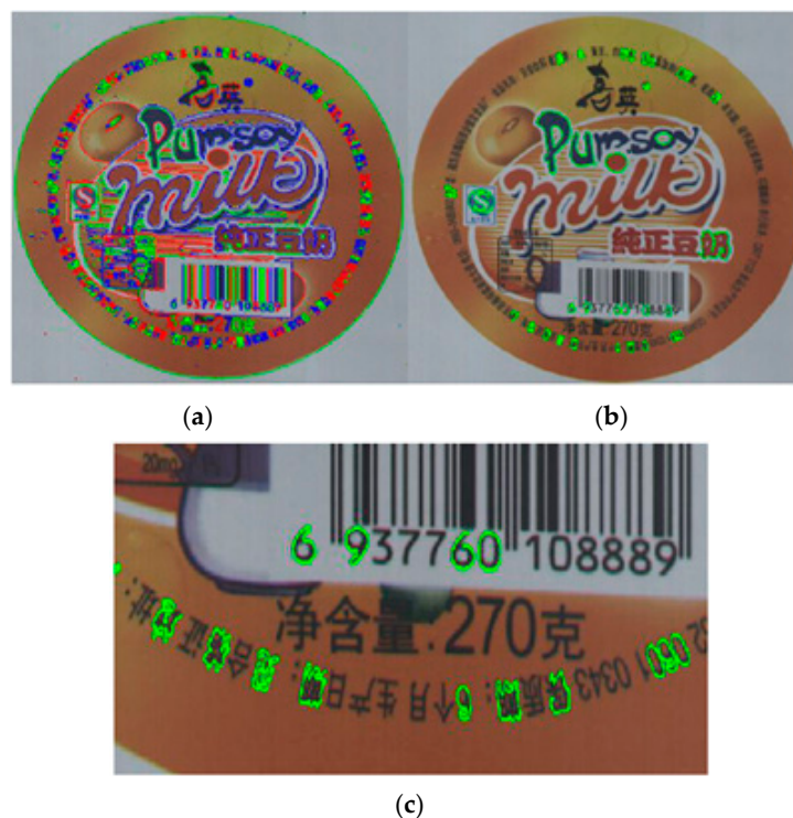
Figure 10. First set of searching results for good shapes. (a) All shapes detected; (b) good shapes searched; (c) partially enlarged image of Figure (b).
