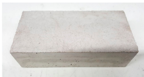
Figure 7. The brick sample with dimensions of 190 × 90 × 57 mm produced using the mixture proportion of ROG in Table 4.
