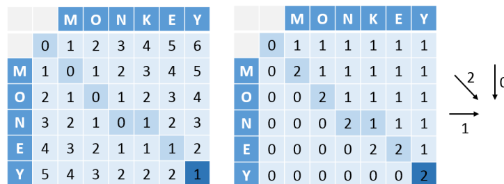
Figure 3. An example of the minimum edit distance algorithm. The left sub-figure show the F matrix, which is the minimum edit distance for the sub-sentences. The right sub-figure shows the path matrix, from which we can get the alignment.
