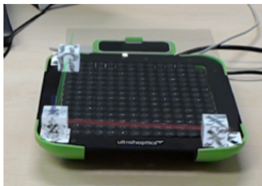
Figure 7. Manual alignment over the Ultrahaptics: The user has positioned three digital cube anchors over three physical stickers.
