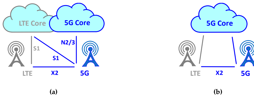
Figure 2. Different 5G interfaces: (a) in early 5G phase; (b) in mature 5G phase.
