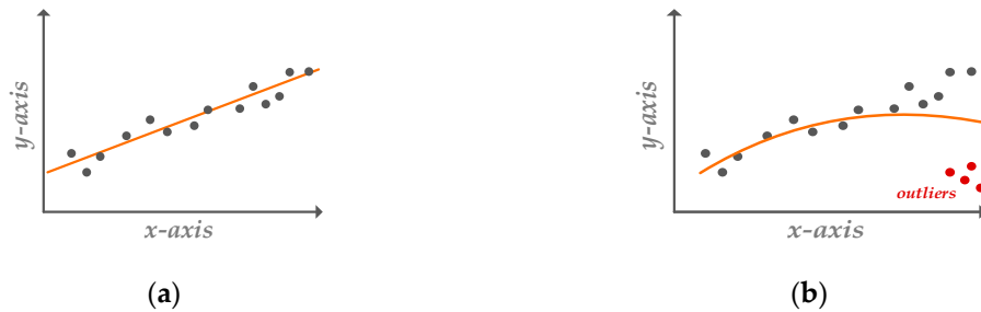
Figure 4. Conventional learning methods may be easily affected by outliers. (a) Common condition; (b) affected by outliers.
