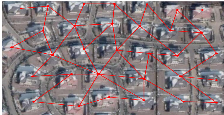
Figure 15. Communication topology of the 32 customers' system.
