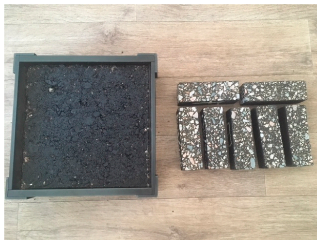
Figure 4. Asphalt concrete samples: in the shape of a square slab with dimensions 305 × 305 × 50 mm (left); in the shape of a rectangular prism with dimensions 5 × 5 × 50 mm (right).
