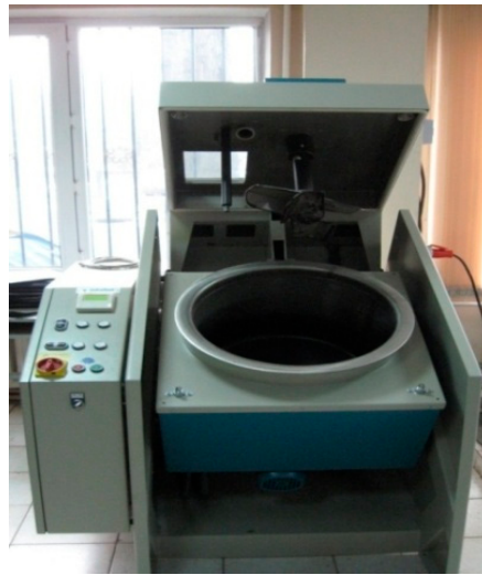
Figure 3. Laboratory mixing device for preparing of asphalt concrete mixes.
