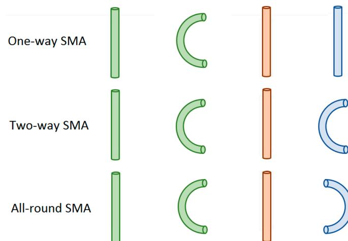
Figure 4. Different SMA shape memory effects.
