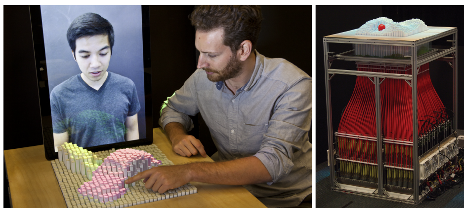
Figure 5. inFORM shape display hardware. The inFORM system actuates and detects shape change using 900 mechanical actuators, while user interaction and objects are tracked with the help of an overhead depth camera. A projector provides additional visual feedback [24,25].
