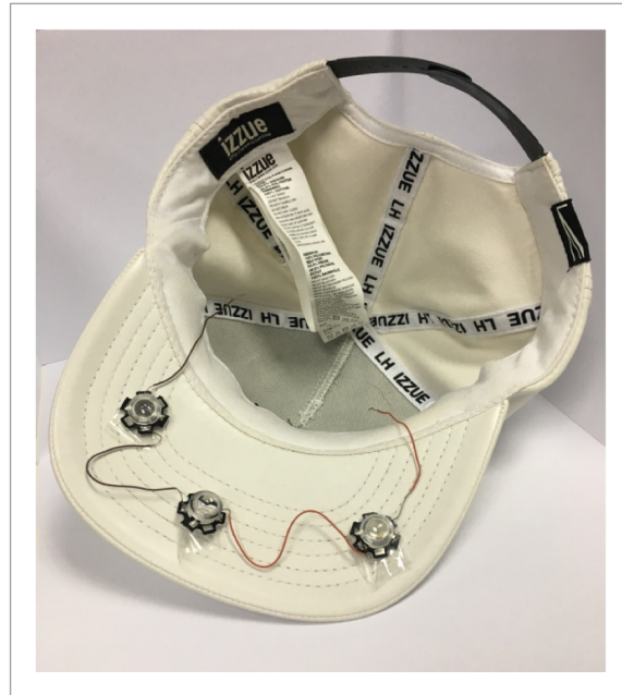
Figure 14. The cap with some infrared LED (Image Credit: Zhou et al. [38]).
