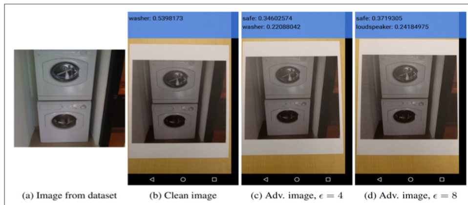
Figure 10. Demonstration of a black-box attack on a phone app for image classification using physical adversarial examples (Image Credit: Akhtar et al. [80]).
